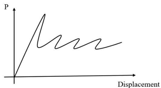
**Figure 1.3** Illustration of sequential buckling behaviour
