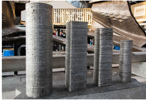
Figure. 10 As-printed components by WAAM and without surface polish (Buchanan & Gardner, 2019)
