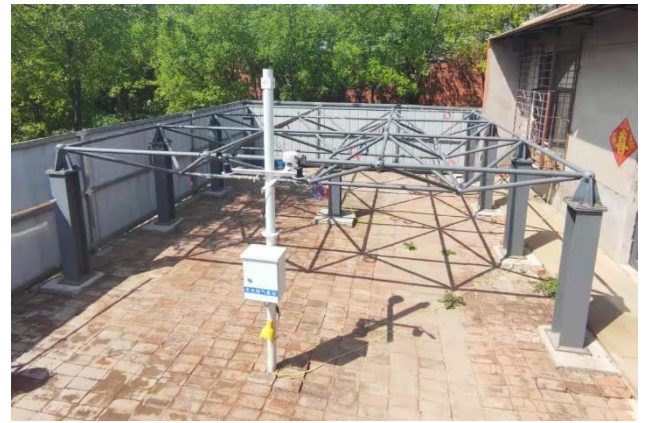
FIGURE 3. The experimental spatial grid structure.
