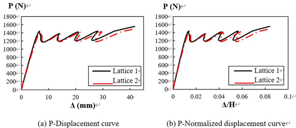
**Figure 9** Load displacement response for lattice 1 and lattice 2
