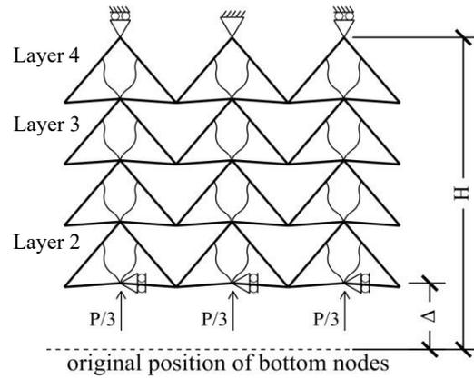
**Figure 8** Theoretical load and boundary condition
