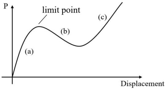
**Figure 2** Illustration of snap-through behaviour
