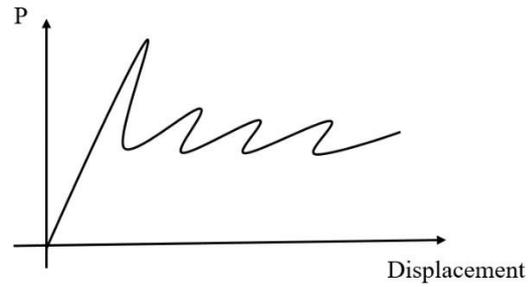
**Figure 3** Illustration of sequential buckling behaviour
