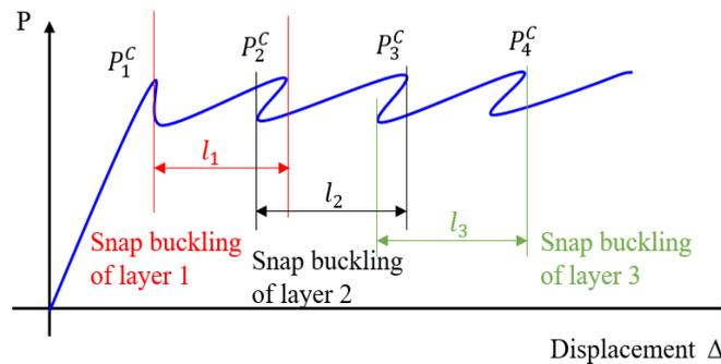
**Figure 4** Illustration of the approximate quasi-zero stiffness range
