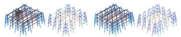
Comparing the results, it can be deduced that the exoskeleton is more stressed in the case of the structure with collaborating wall, which is another reason that lead to analyze the Benchmark System in detail.
