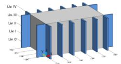
Exoskeletons are shear walls made from metallic material. Their operation can be 2D or 3D and, in the 2D case, the walls can be arranged orthogonal or parallel to the building facades. In particular, this work refers to 2D systems orthogonal to the plan of the reinforced concrete building to be retrofitted. But what are the advantages and disadvantages of exoskeletons?
