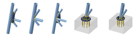
The local analysis of the nodes is very important to better capture the stress distribution at the nodes. In fact, independently of the  $\zeta_E$  to be achieved, it can be observed that the material S275, as previously mentioned, is not sufficient in strength because there are large areas of concentrated stress which plasticize the node. In case of S355, the members have a lower work rate such that steel doesn't reach yield strength.
