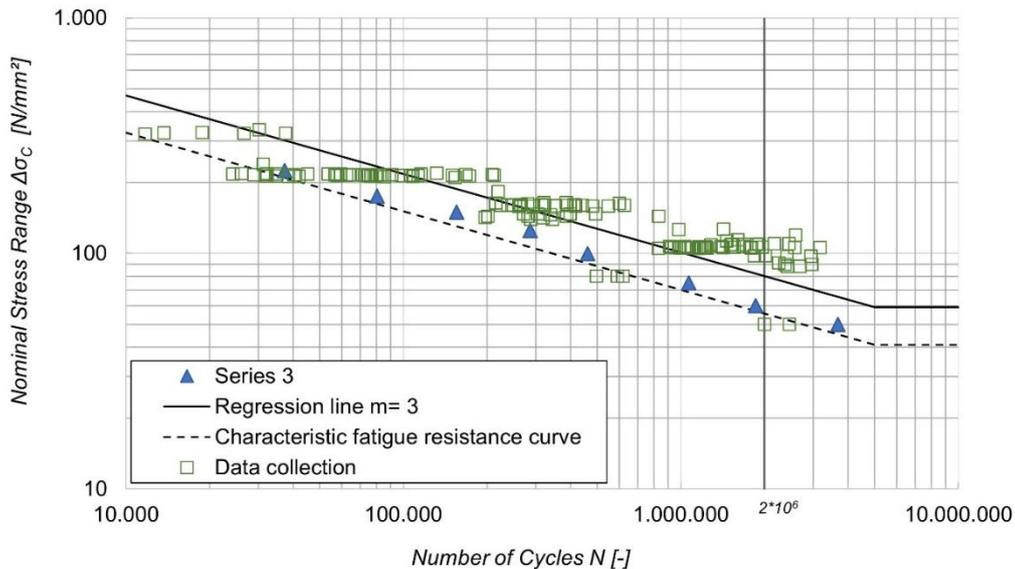
**Figure 4: Overall evaluation of tubular bracings with an inclined sealing plate (without fillet weld).**
