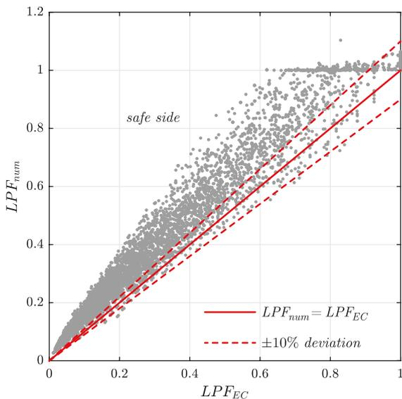
Fig. viii: Results (LPF: Load proportionality factor) of the GMNI-analysis showing the decisive results of the individual subpanel and stiffened panel, considering the proposals of POUROSTAD and a magnification factor of  $f_\lambda = 1,3$  for increasing the global slenderness  $\lambda_p$ .
