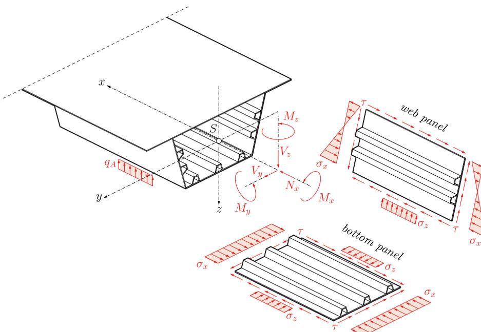
Fig. ii: Box girder with the loads due to bending and the locally applied reaction force  $q_A$  [3].
