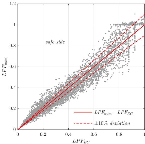
Fig. vii: Results (LPF: Load proportionality factor) of the GMNI-analysis showing the decisive results of the individual subpanel and stiffened panel, considering the suggestions of POUROSTAD.
