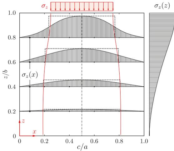
Fig. iii: Stress distribution  $\sigma_z(z)$  and  $\sigma_z(x)$  of the analytical solution as a function of the loading length ratio of  $c/a = 1/2$ . The aspect ratio of the plate is  $\alpha = 1,0$ .
