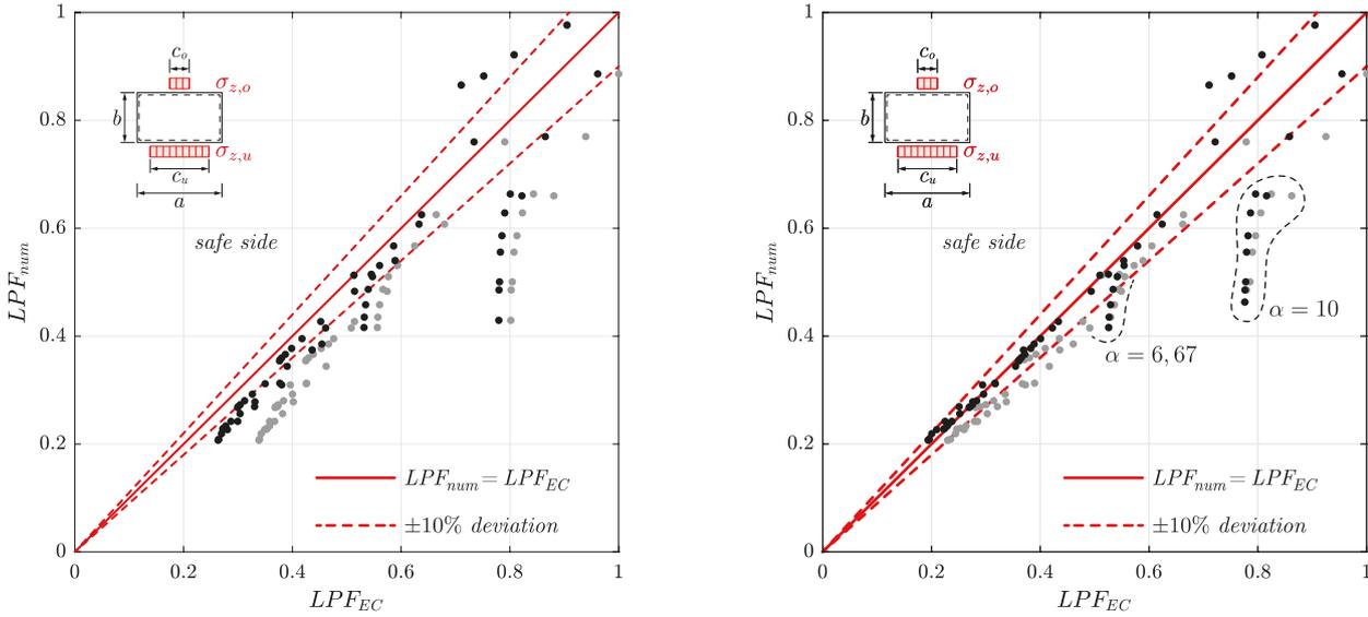
Fig. v: LPF (Load proportionality factor) of the GMNIA without (left) and with (right) using Eq. (6.14) according to prEN 1993-1-5. Furthermore, the scattered points shows the use of the interpolation function proposed by Pourostad (●) and according to prEN 1993-1-5 section 6.6.1 (◐).
