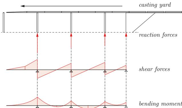
Fig. i: Schematic representation of the incremental launching method with the reaction forces and the shear and bending moment distributions.
