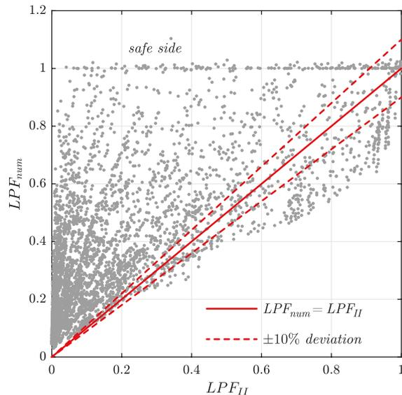
Fig. vi: Results (LPF: Load proportionality factor) of the longitudinal stiffener according to the second order analysis (prEN 1993-1-5).
