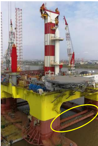
Figure 1: Semi-submersible drilling platform (left) and semi-submersible crane vessel (right) [1], bracings highlighted in yellow
