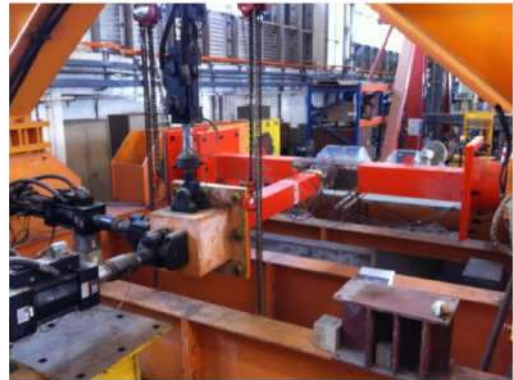
Figure 118: Zhao et al. fatigue test specimen (left) and test set-up (right)
