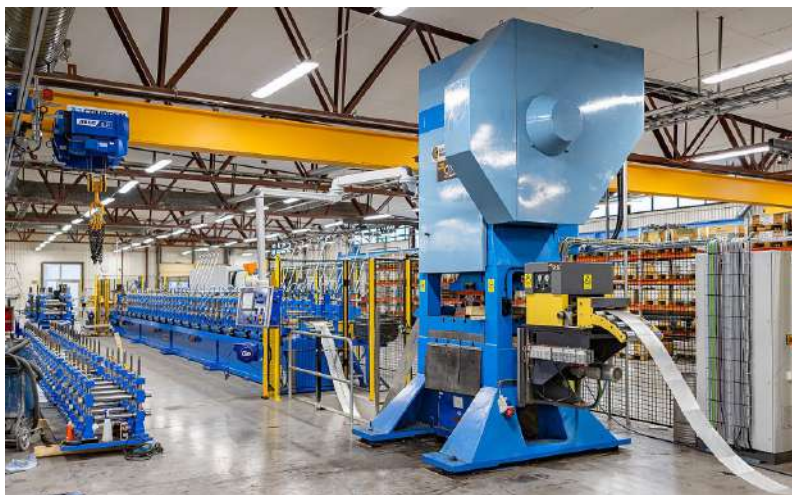
Figure 2.2: Roll forming production setup at Bendiro.
