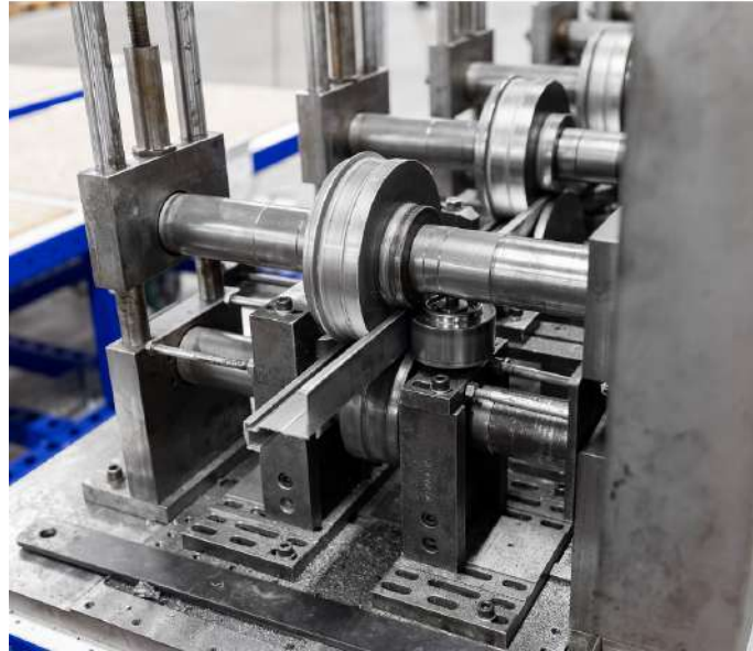
Figure 2.3: Roll forming production machines at Bendirol.
