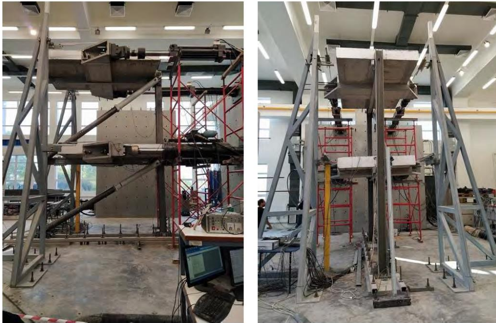
Figure 3-11 General setup of the 2D structure
