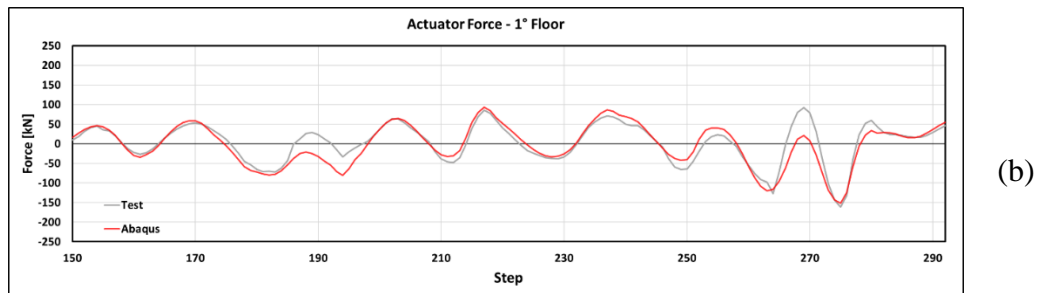
Figure B1-2 Actuator Force: (a) Second Floor; (b) First Floor
