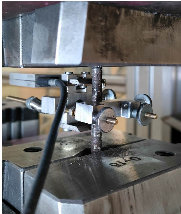
Figure 6.34 Experimental tensile test setup in case of WAAM single bars specimens.
