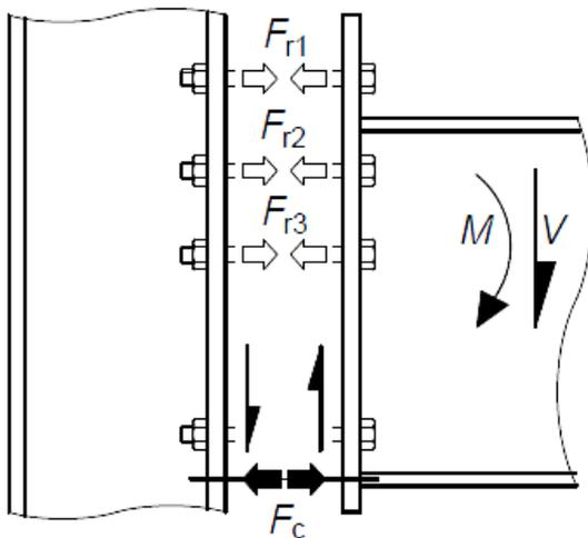
Fig 36a: Forces in an end plate connection
