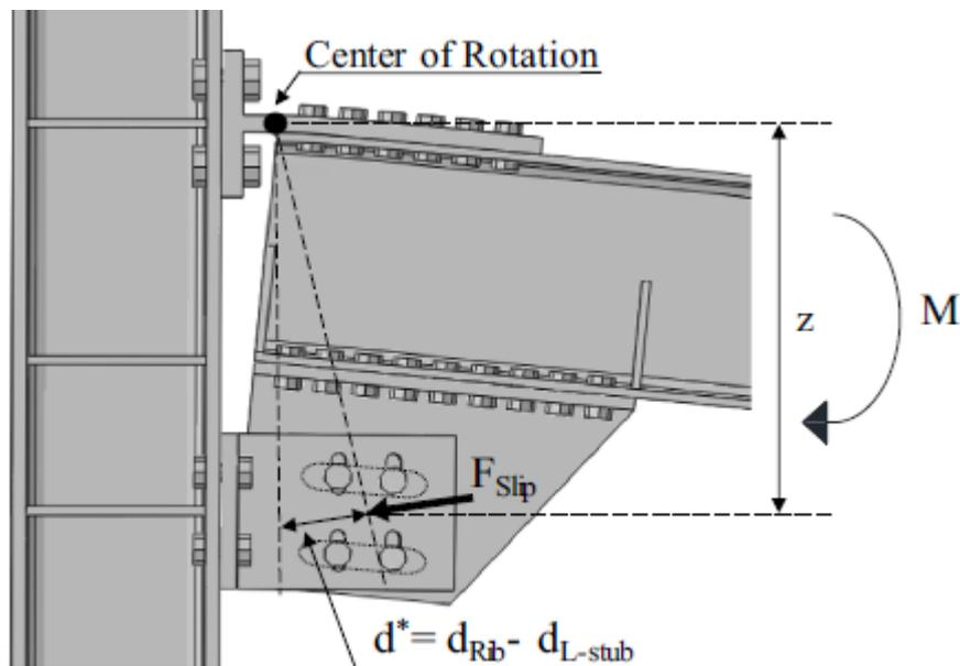
Fig 6: Side view of the FREEDAM joint in action
