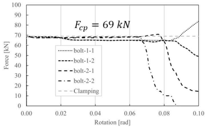
Fig 20: (Sagging) Evolution of the Preload Force in the damper bolts
