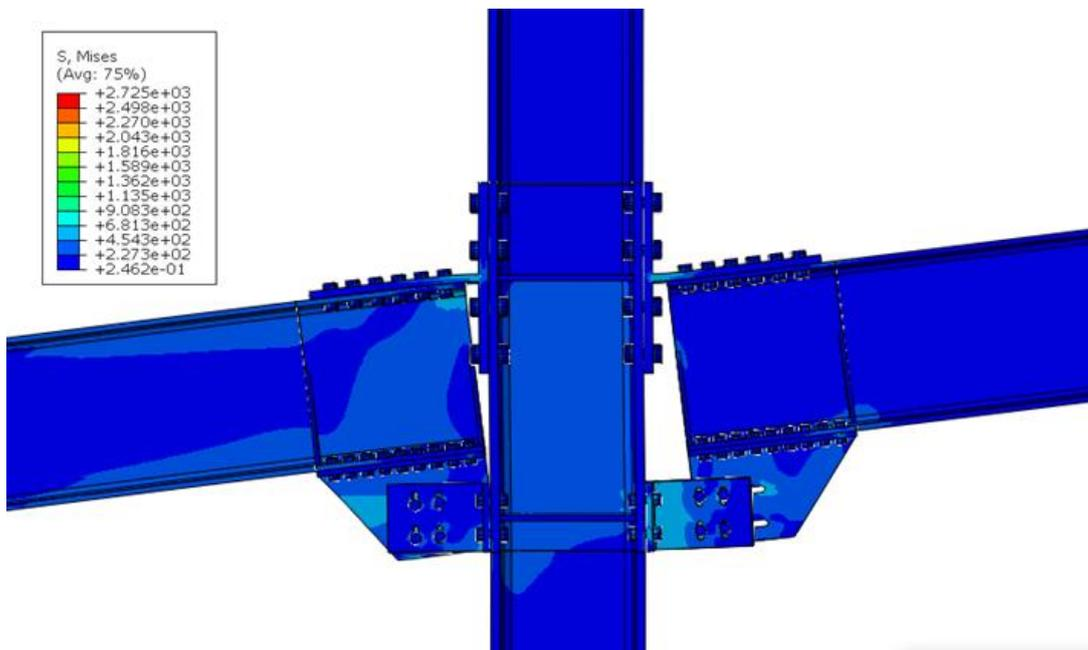
Fig 46: Von Mises stress distribution
