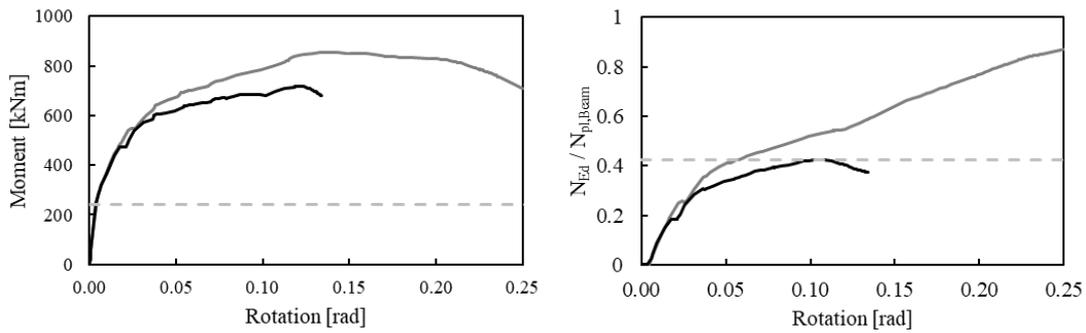
Fig 55: Bending moment – rotation diagram (on the left) and catenary axial load on the right. Previous design Y-II-XJ (in black) and proposed design Y-II-XJ-MOD (in grey)
