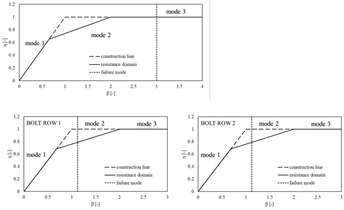
Fig 54: Column equivalent T-stub resistance domain: previous design (top) and proposed design (bottom)
