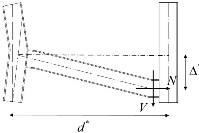
Fig 15: Forces involved in a Column Loss
