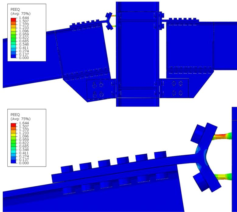
Fig 31: PEEQ distribution, with detail of the T-stub
