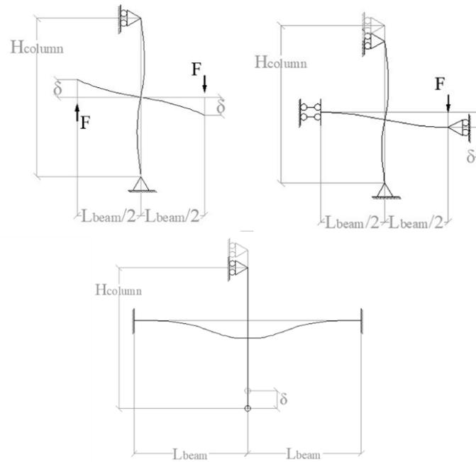
**Fig 11: static schemes for: Seismic Scenario (top left), Hogging Column Loss Scenario (top right), Sagging Column Loss Scenario (bottom)**
