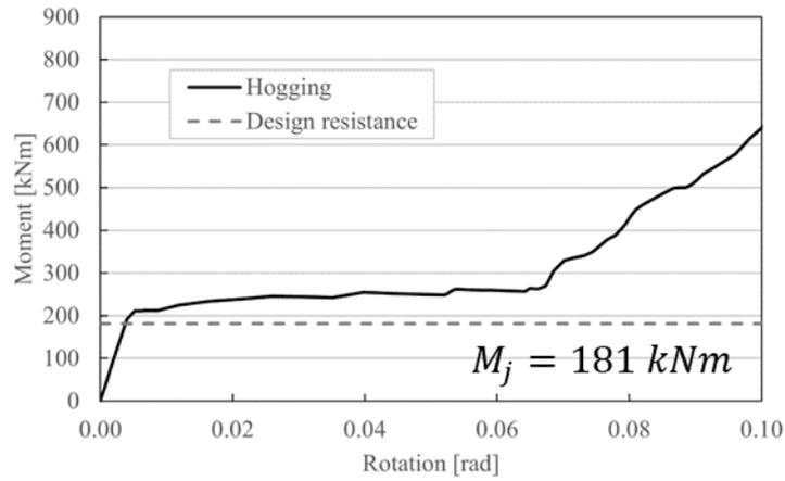
**Fig 17: Hogging bending moment-rotation curve**
