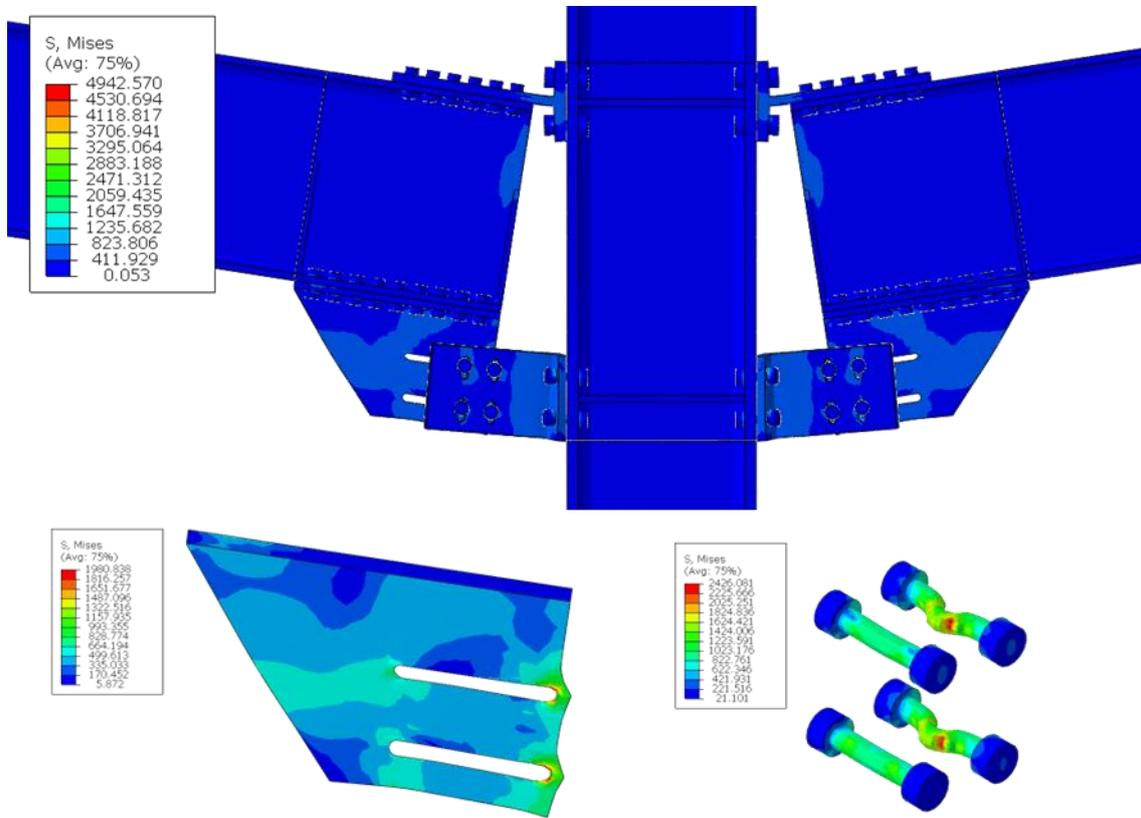
Fig 34: Von Mises stress distribution, with haunch and damper bolts in detail
