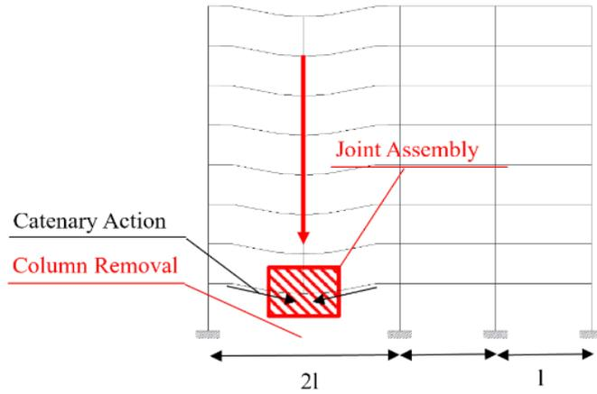
Fig 14: Sagging Column Loss
