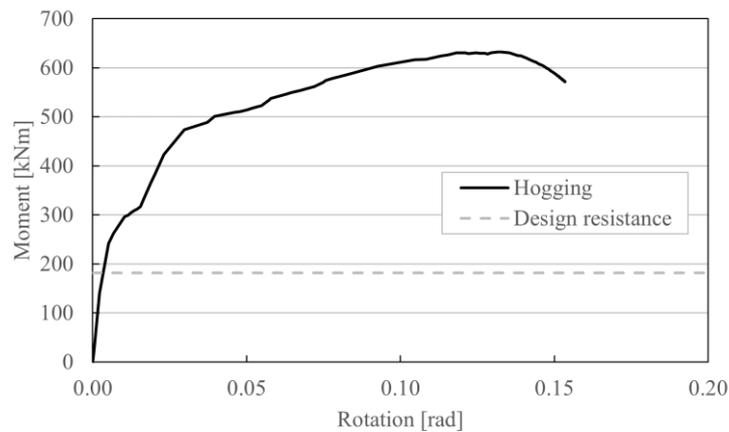
Fig 27: Hogging bending moment-rotation curve
