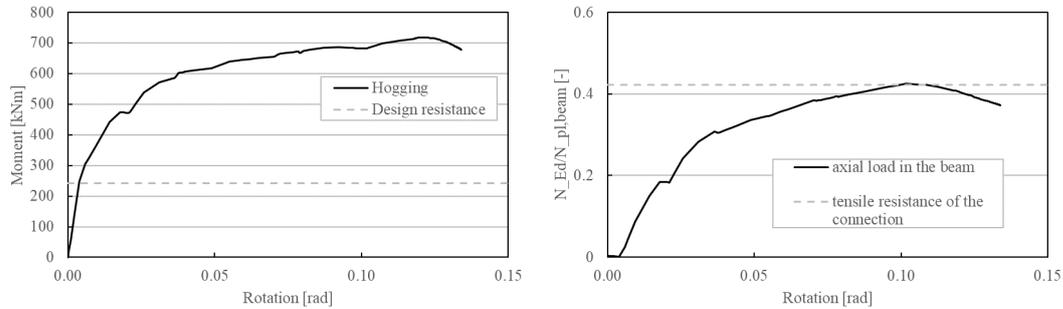
Fig 52: Hogging bending moment - rotation (left), non-dimensional axial load - rotation (right)
