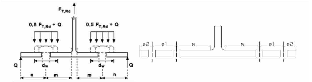
Fig 43: 4-bolts T-stub
