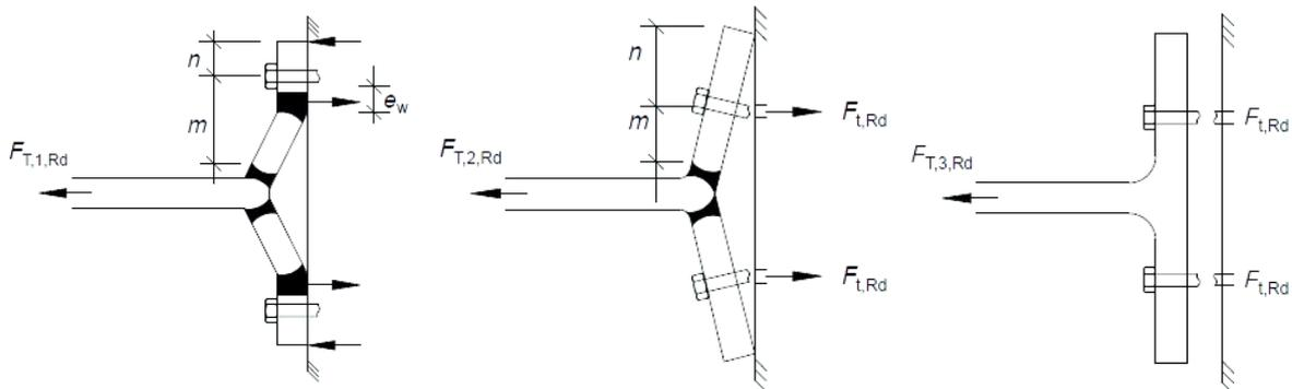
Fig 36b: different mode of failure for a T-stub; mode 1 (left), mode 2 (center), mode 3 (right)
