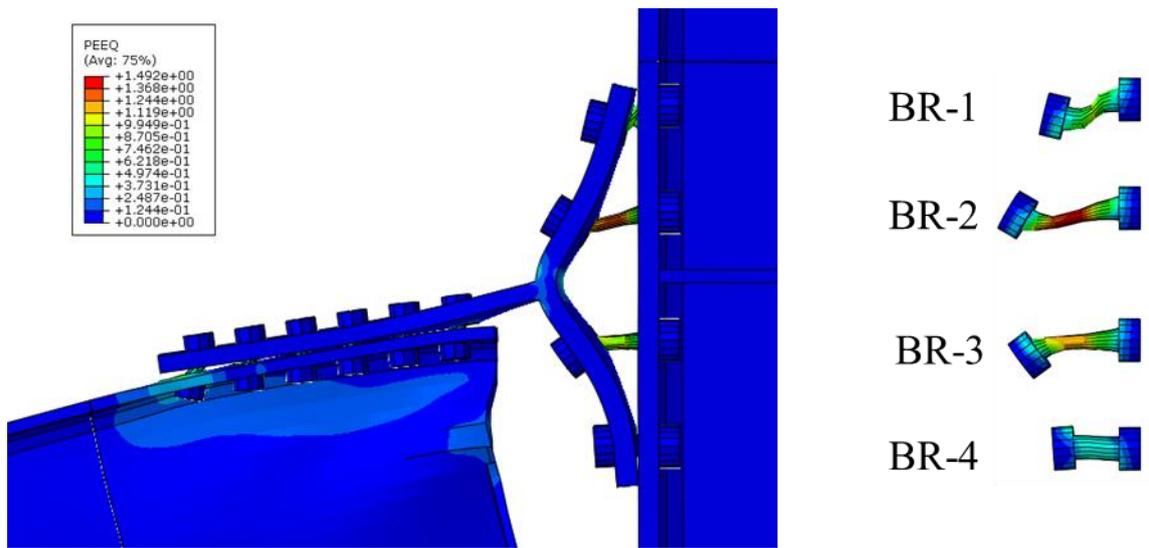
Fig 50: 4-bolts T-stub detail under Column Loss "Hogging"
