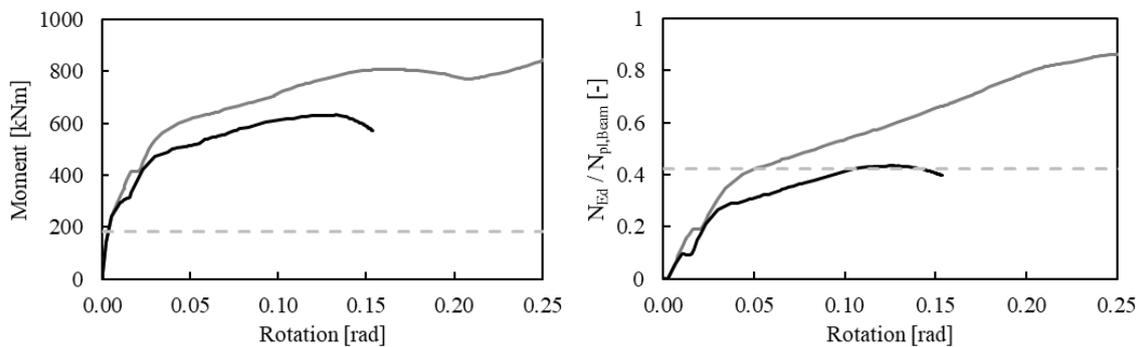
Fig 48: Bending moment – rotation (on the left) diagram and catenary axial load of the X-II-XJ-MOD the previous joint (in black) is confronted with the new version (in grey)
