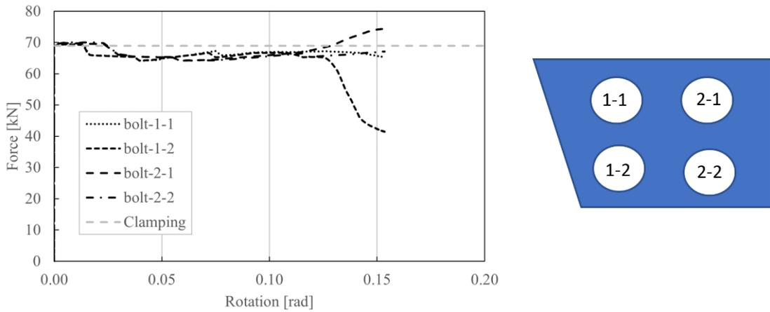
Fig 29: (Hogging) Evolution of the Preload Force in the damper bolts; damper bolts nomenclature (right)
