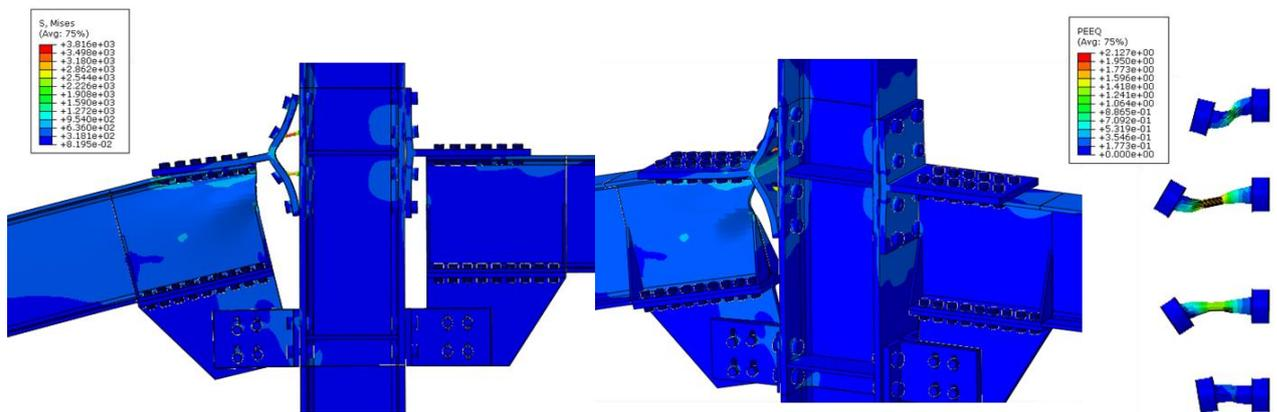
Fig 56: Von Mises stress distribution (left) and PEEQ distribution (right)
