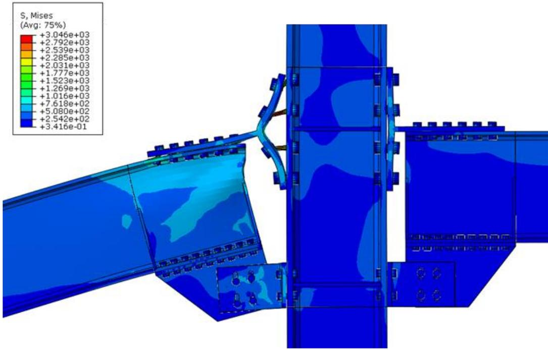
Fig 49: Von Mises stress distribution
