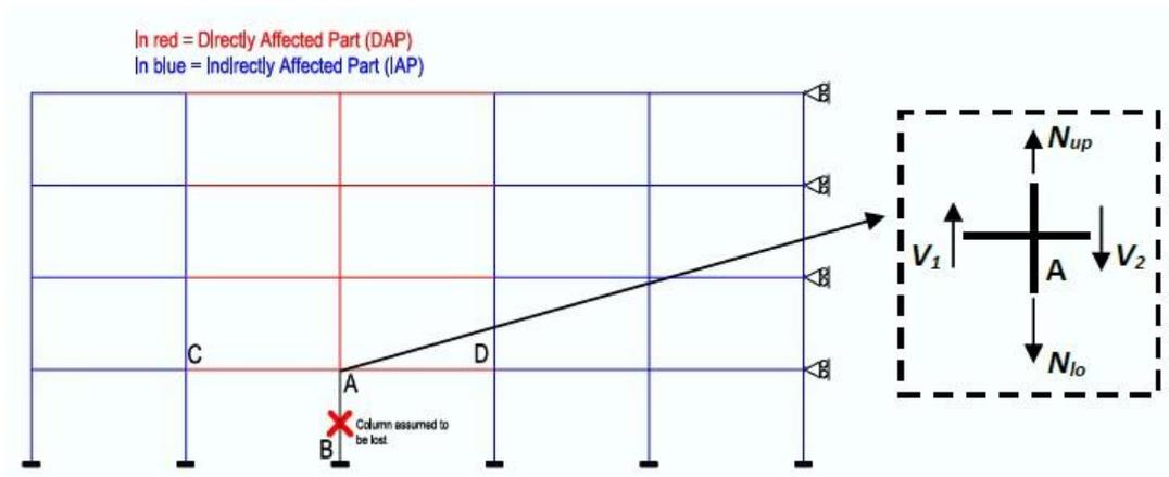
Fig 12: Directly Affected Part and Indirectly Affected Part of a Column Loss Scenario
