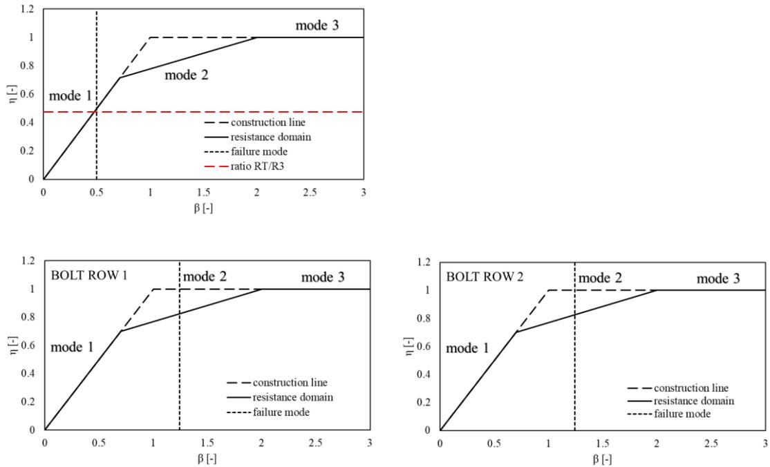
**Fig 44: joint X-II: T-stub flange behaviour (up-left), column side bolt row 1 (bottom-left), column side bolt row 2 (bottom-right)**
