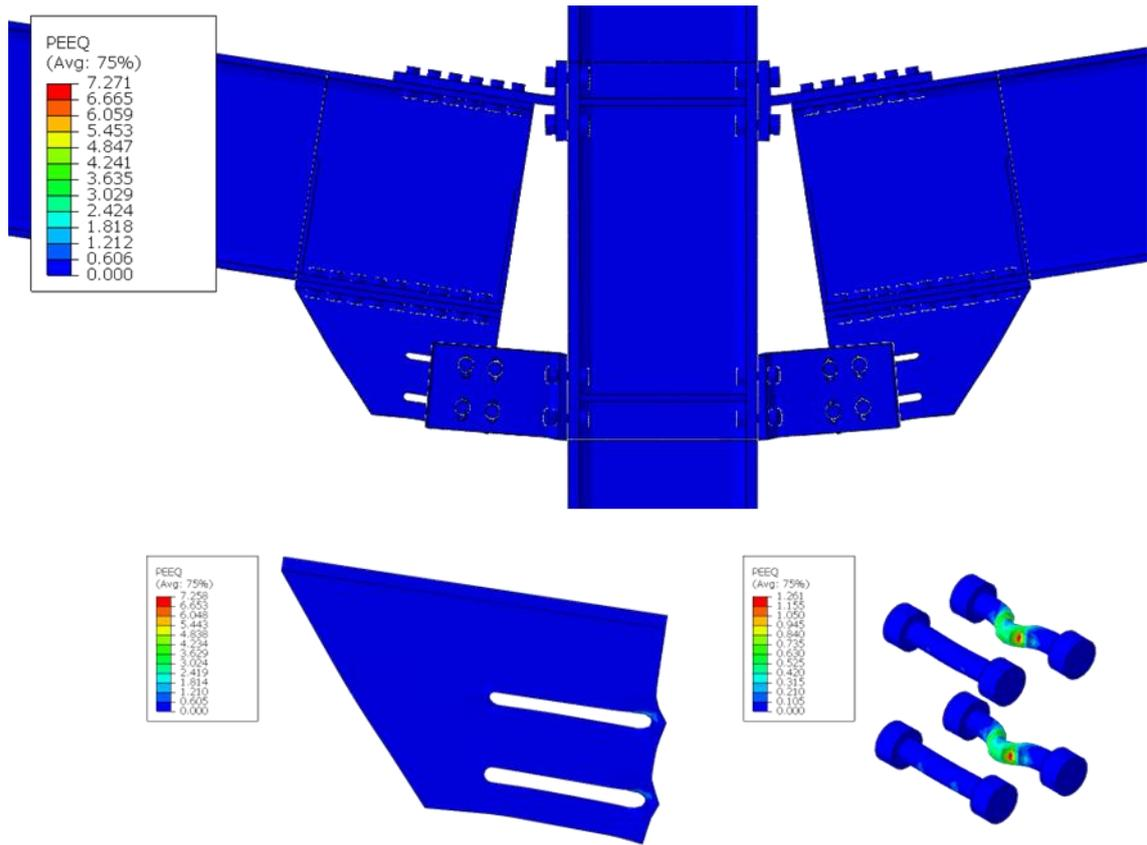
Fig 35: PEEQ distribution, with haunch and damper bolts in detail
