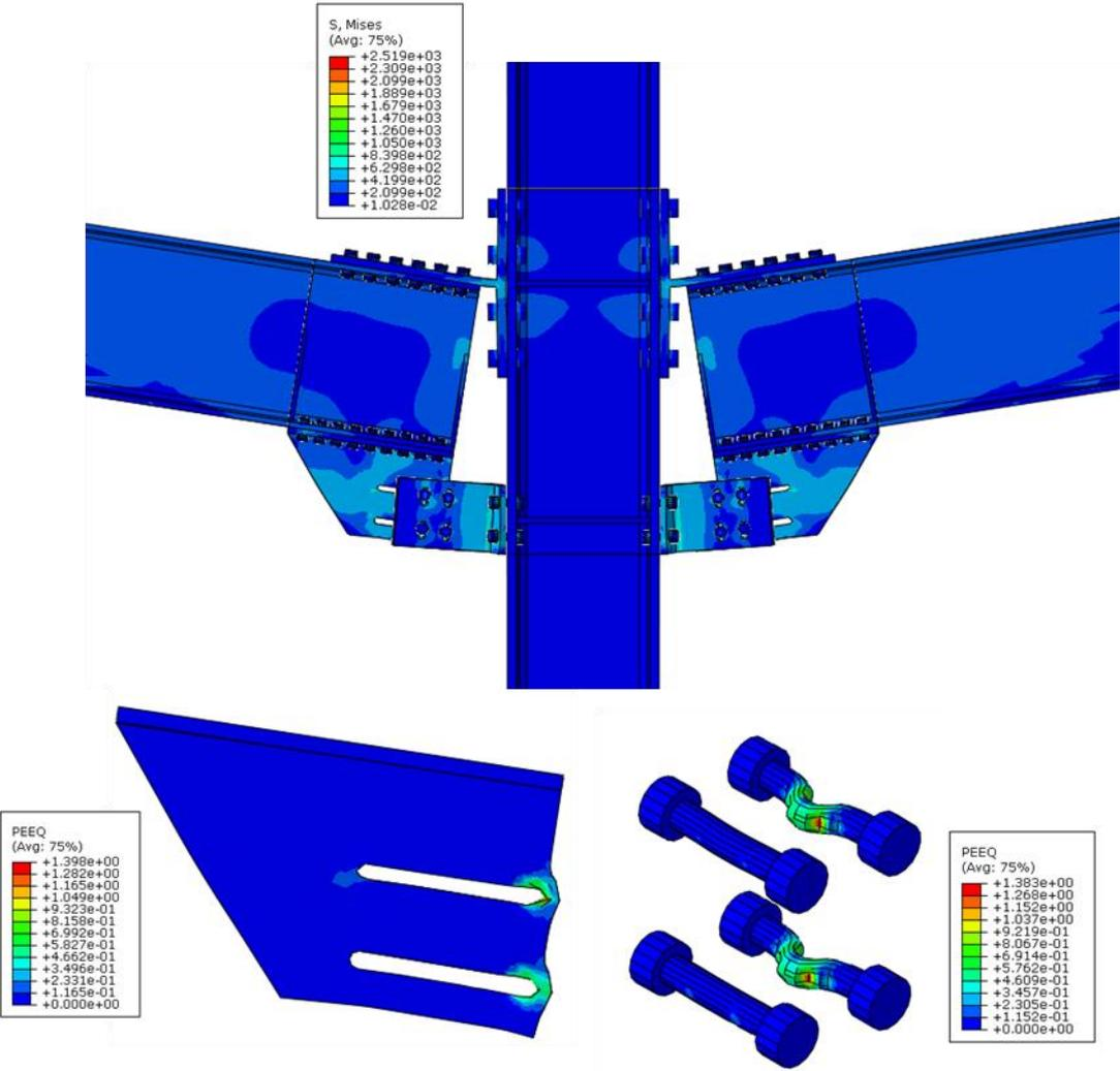
Fig 51: Von Mises stress distribution (top); PEEQ distribution on the haunch and damper bolts (bottom)
