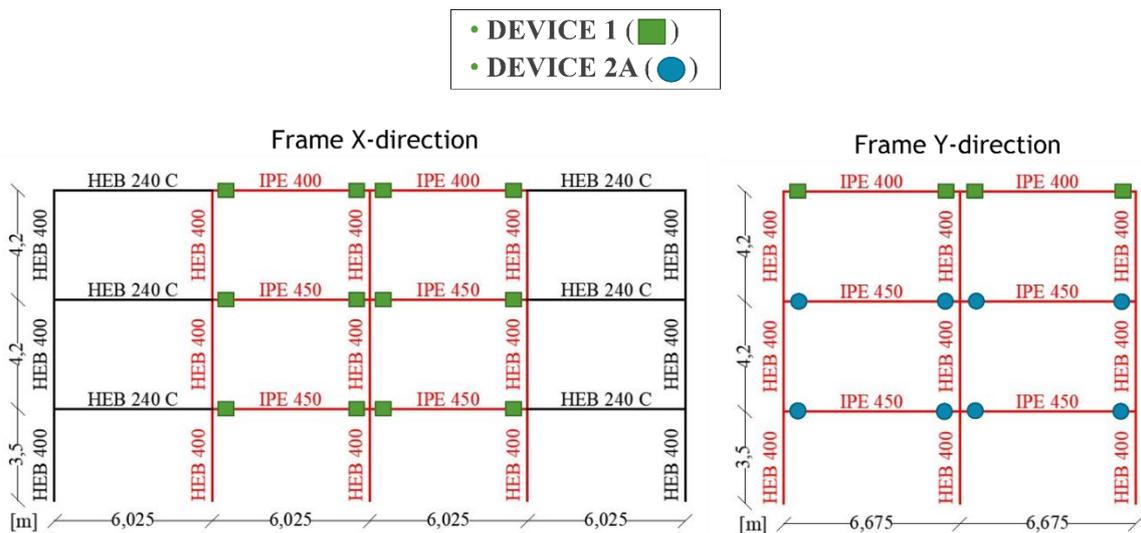
Fig 10: details of the X-MRF (left) and Y-MRF (right), with FREEDAM devices location
