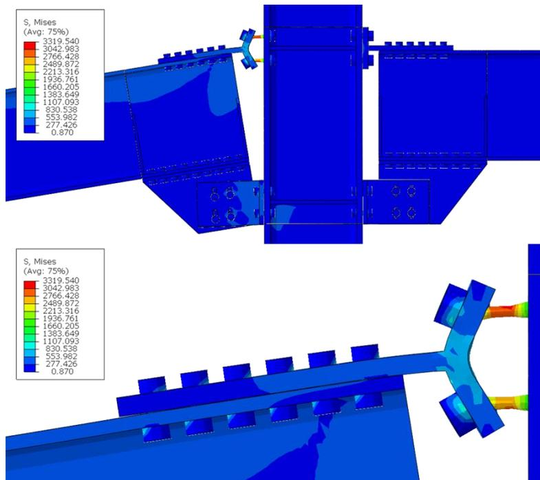
Fig 30: Von Mises stress distribution, with detail of the T-stub
