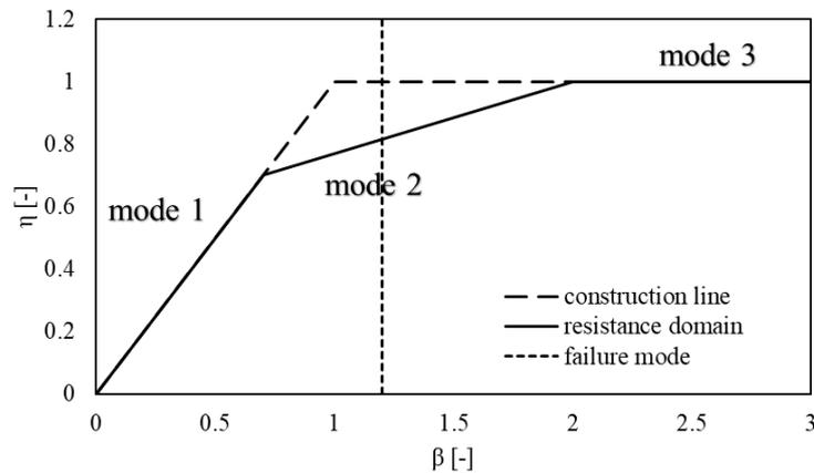
Fig 41: Resistance domain for T-stub flange
