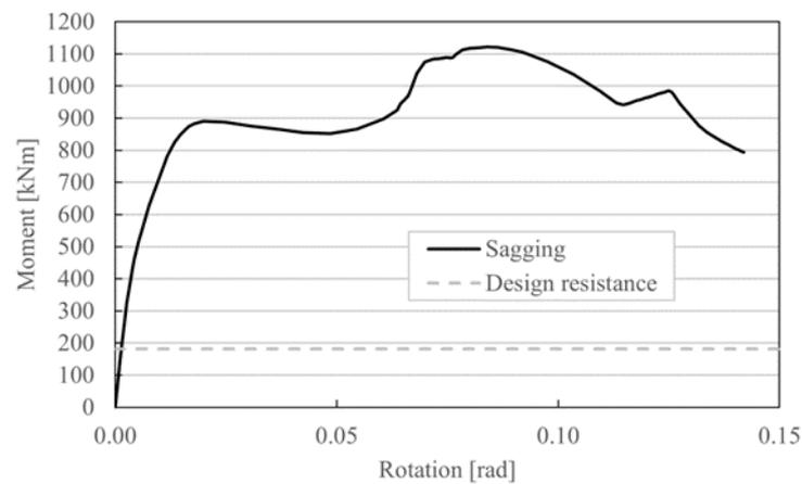
Fig 32: Sagging bending moment-rotation curve
