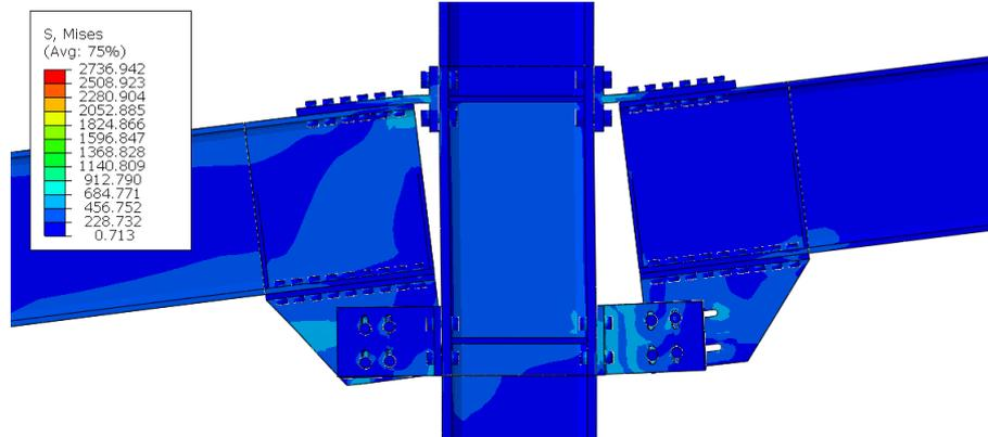
Fig 22: (Hogging) Von Mises stress distribution
