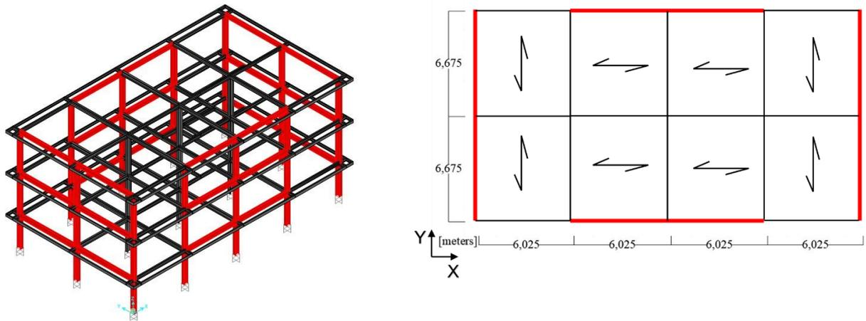
Fig 9: 3D view of the structural elements (left); plan view, with MRF bays in red (right)
