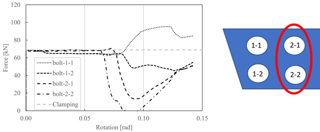
Fig 33: (Sagging) Evolution of the Preload Force in the damper bolts
