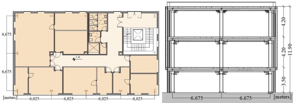
Fig 8: plan view (left) and elevation view of the Y-MRF (right)
