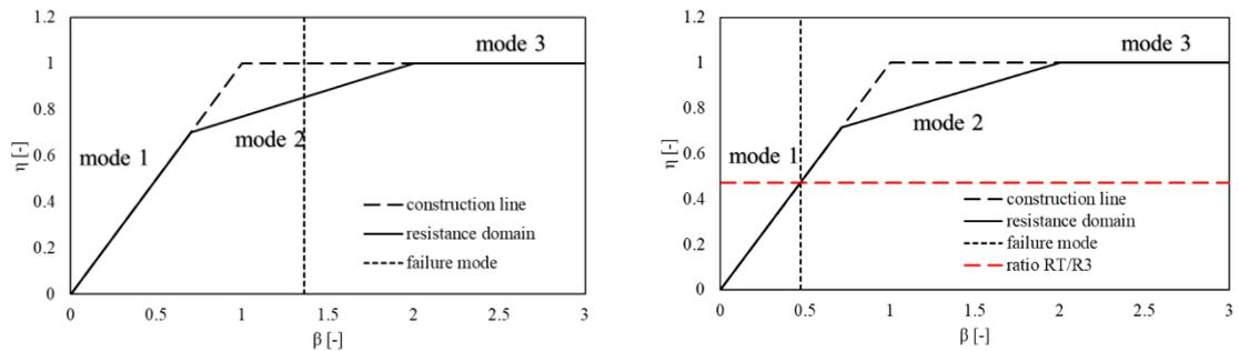
Fig 53: T-stub flange resistance domain: previous design (left) and proposed design (right)
