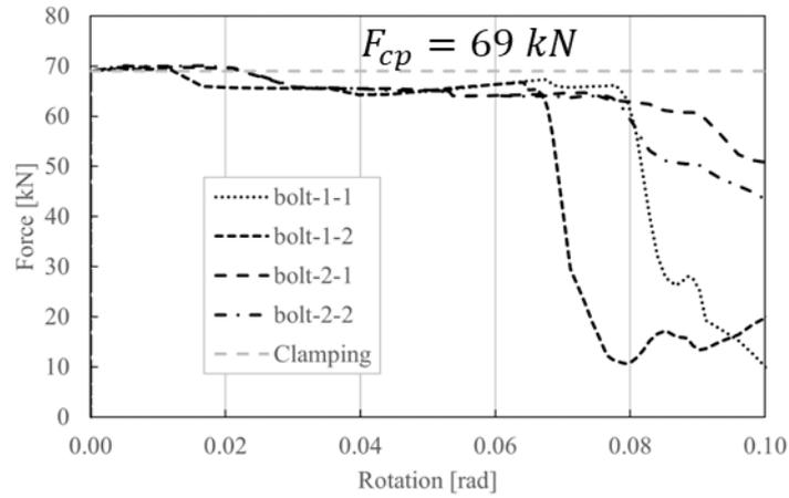
Fig 19: (Hogging) Evolution of the Preload Force in the damper bolts
