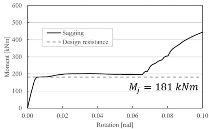
**Fig 18: Sagging bending moment-rotation curve**
