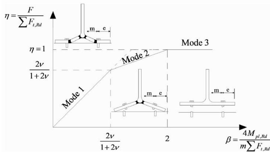
Fig 38: T-stub resistance and corresponding mechanism according to EN1993:1-8
