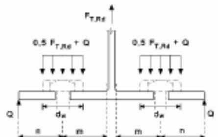
**NOTE 1:** In bolted beam-to-column joints or beam splices it may be assumed that prying forces will develop.
