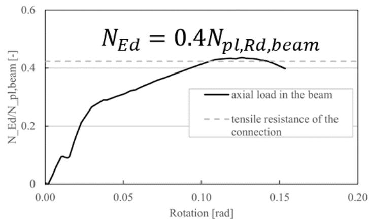
Fig 28: non-dimensional axial load on beam
