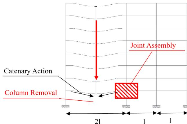
Fig 13: Hogging Column Loss
