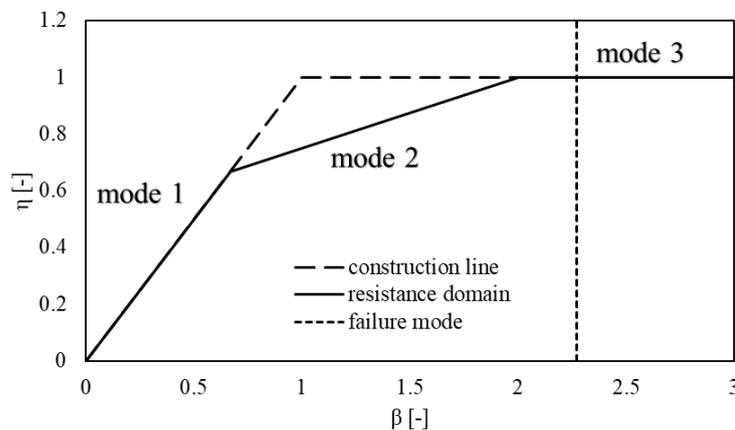
Fig 42: Resistance domain for column flange
