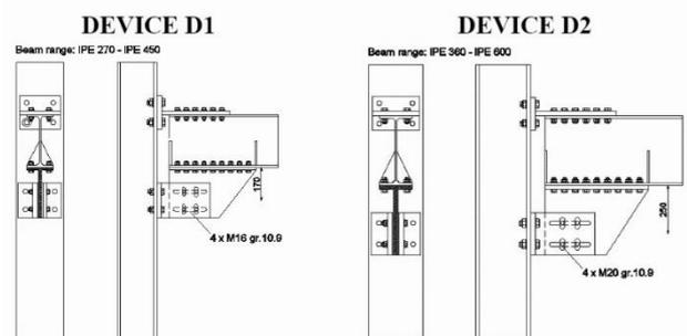
Fig 3: Prequalification table for the FREEDAM devices (left); FREEDAM devices to be used in the DREAMERS building (right)
