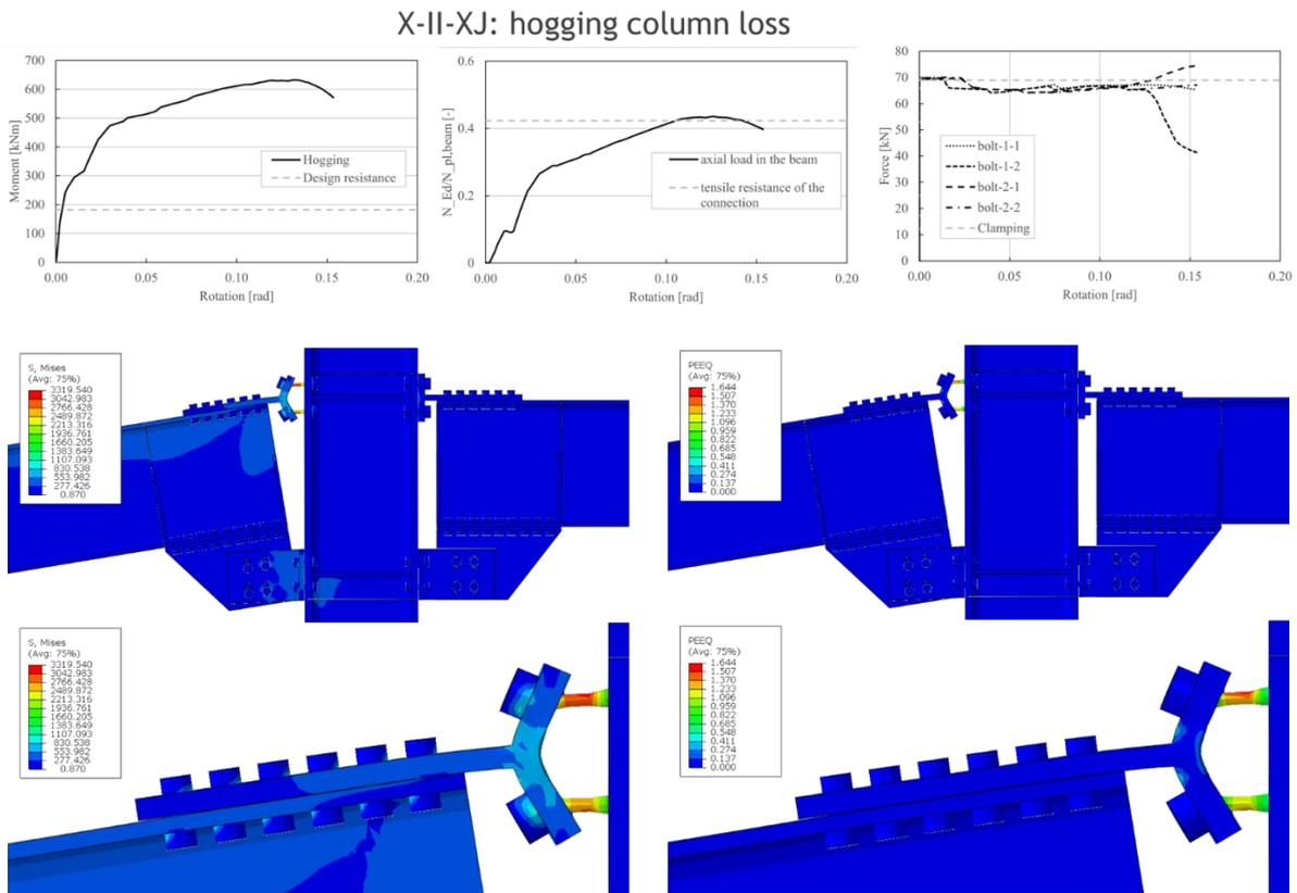
In case of **Positive Moment induced by Column Loss** the situation is analogous, the failure is localized in the shank of the damper bolts, when they come into contact with the stiffening plate.
