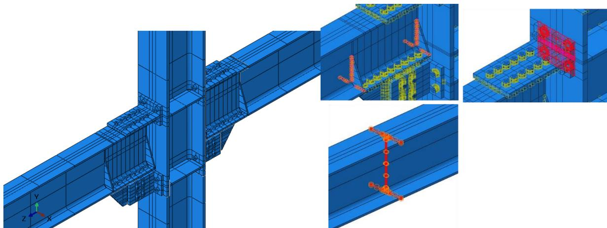
Fig 6: X-joint as modelled in the FE software (left), interactions, rigid body constraints, tie constraints (right, clockwise)
