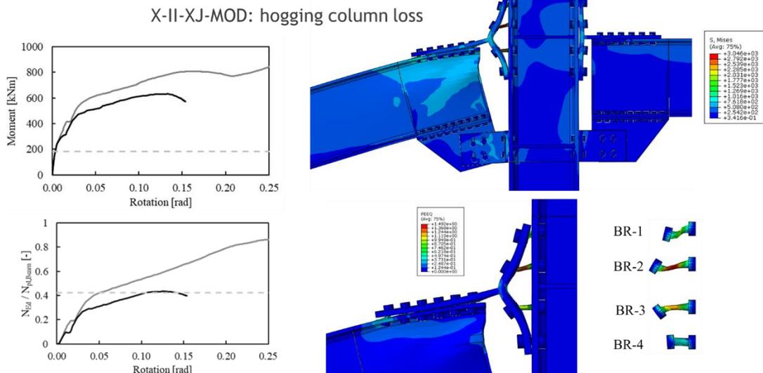
The reinforced joint has the same seismic behaviour as the original joint; therefore, all considerations made about FREEDAM joints previously are still valid.
