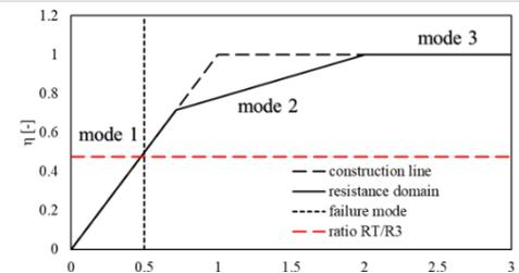
Fig 8: Resistance domains of the T-stub: before (up) and after the proposed modification (down)
