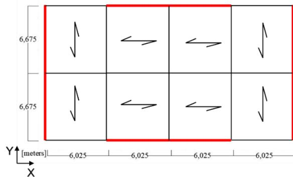
Fig 2: Plan view of the DREAMERS building; MRFs are highlighted in red
