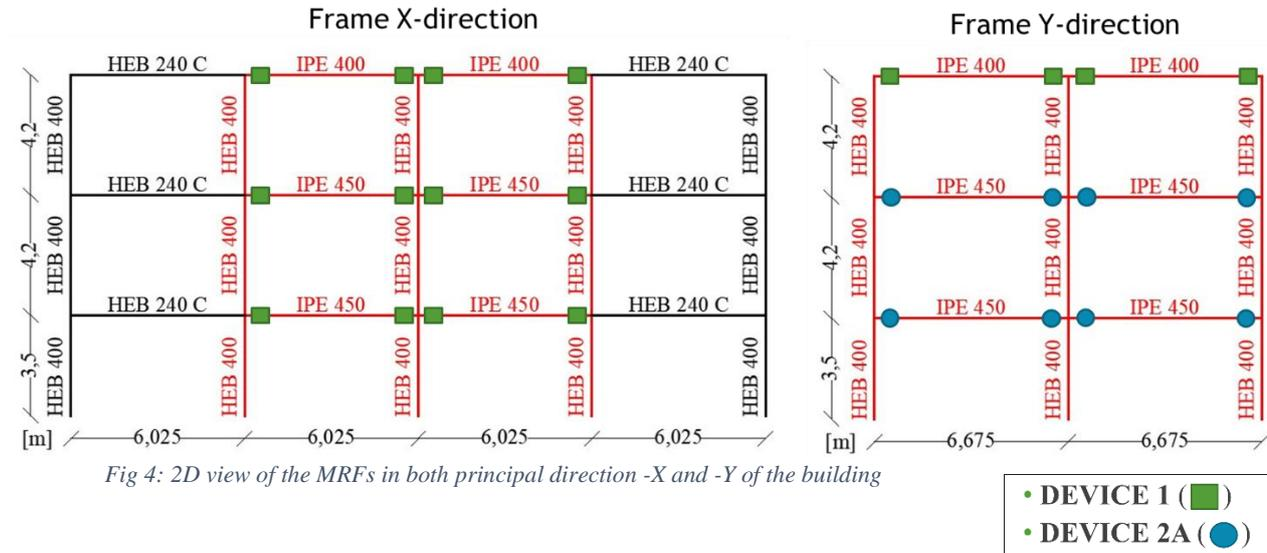
Fig 4: 2D view of the MRFs in both principal direction -X and -Y of the building
