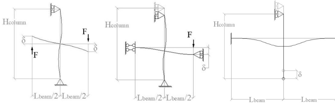
Fig 7: Boundary conditions of each Scenario: Seismic Scenario (left), Column Loss with hogging bending moment (middle), Column Loss with sagging bending moment (right)
