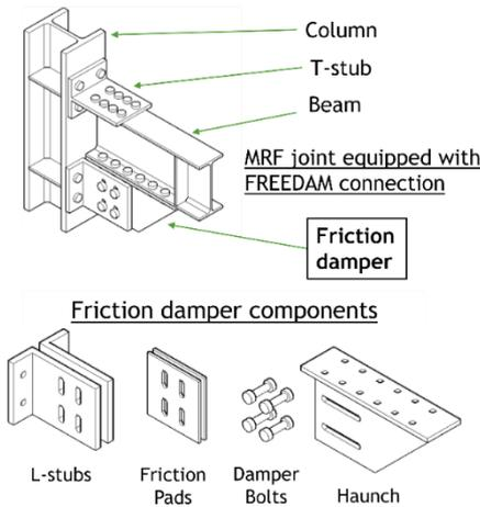
Fig 1: FREEDAM connection and its components
