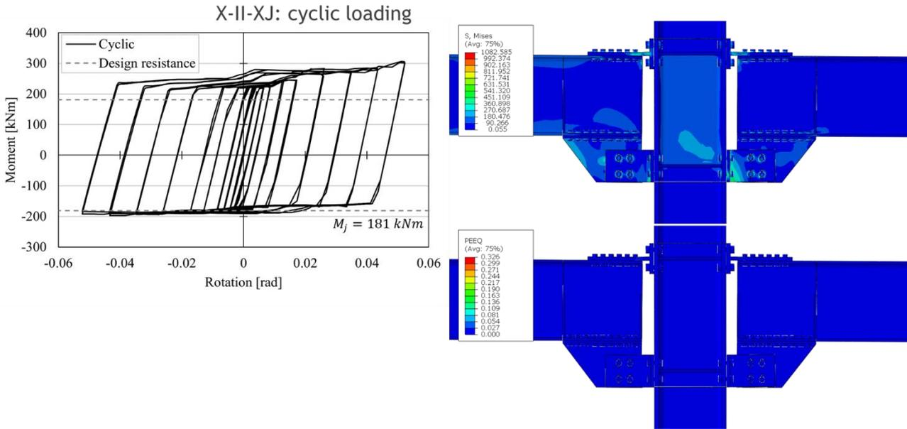
In case of **negative Moment induced by Column Loss** the catenary action on the joint can be observed (diagram in the middle). It is immediate to notice that the upper T-stub undergoes a mode-2 crisis, with partial plasticization of the flange and breakage of the shank of the four connecting bolts (2 bolts per row). Therefore, it was necessary to redesign the T-stub, to guarantee a more ductile failure type and a higher rotational capacity.
