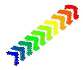
Figure 49 Point cloud cross-sectional segments perpendicular to the main longitudinal axis
