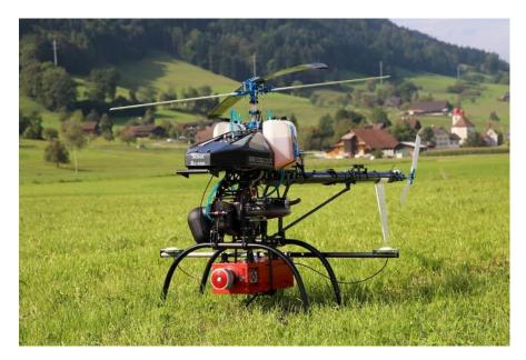
Figure 30 UAV drone with Riegl VOX1 LiDAR scanner
