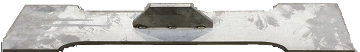
Figure 25. Investigated joint with tack welds.
