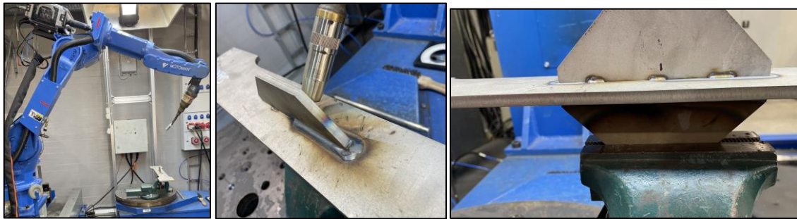
Figure 26. Welding set-up and clamping of specimen.
