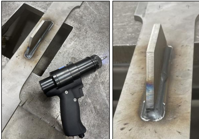
Figure 28. HFMI post-processed weld toes and equipment.
