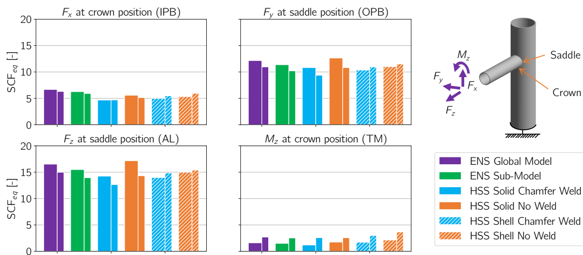
Figure 4.7: Equivalent SCFs for the T-joint. The thick and thin bars represent the SCF at the chord and brace side respectively.
