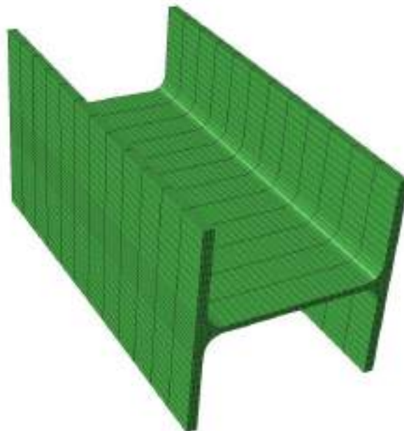
Figure 31: Illustration of the chosen mesh pattern in Abaqus
