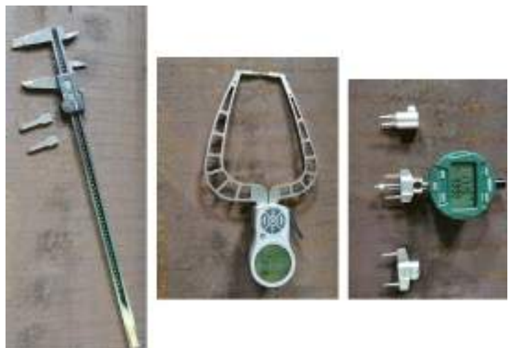
Figure 14: Caliper, electronic quick probe and radii measurement device
