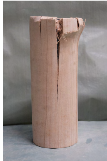
Figure 3.14: S-ST-0 after compression
