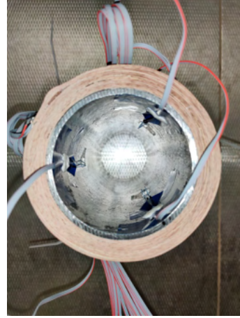
Figure 2.34: DMS-placement in S-ST-0
