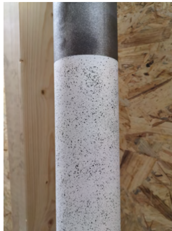
Figure 2.29: DIC surface L-S-0
