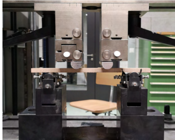
Figure 2.5: Setup four-point bending test
