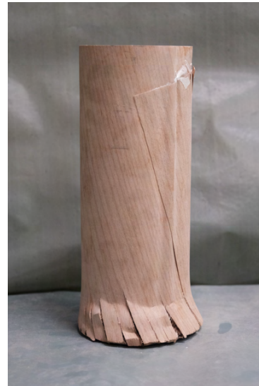
Figure 3.16: S-ST-15 after compression
