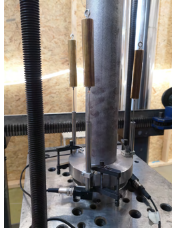
Figure 2.36: Position vertical LVDT
