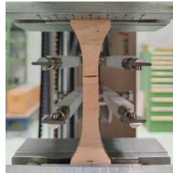
Figure 3.7: Failure of perpendicular sample
