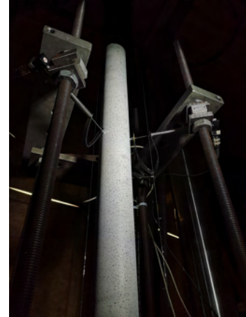
Figure 2.37: Position horizontal LVDT
