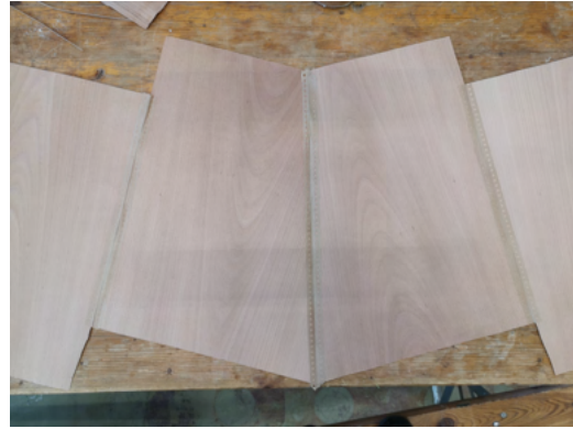
Figure 2.13: Connection of inclined veneer
