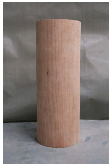
Figure 3.18: S-T-0 after compression
