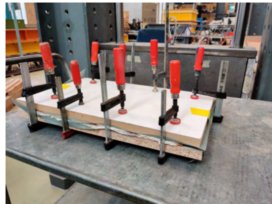
Figure 2.1: Application of glue on the veneer Figure 2.2: Compression of timber veneer plate
