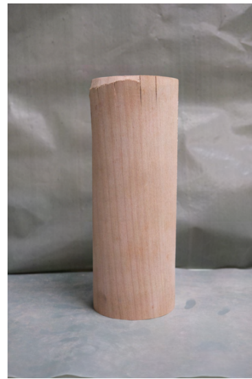
Figure 3.20: S-T-15 after compression
