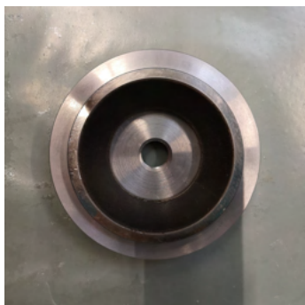
Figure 2.30: Bottom part of hinge
