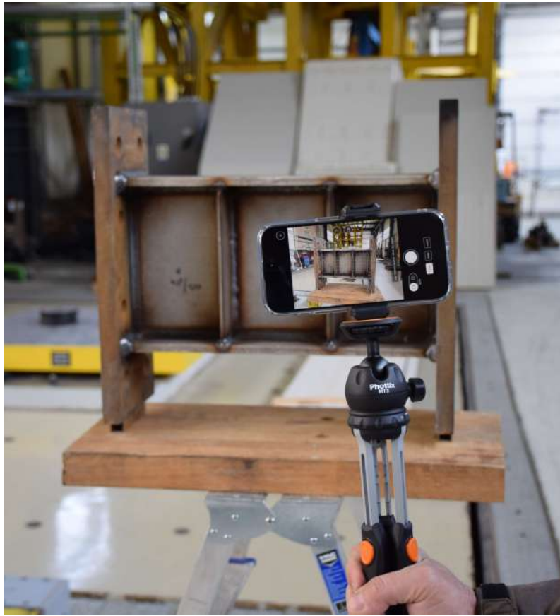
Figure 78 – Smartphone LiDAR measurement set-up
