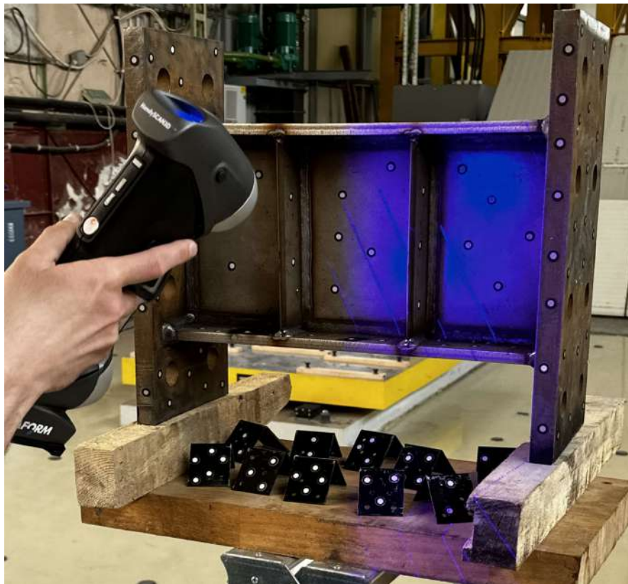
Figure 70 – Re-usable targets for multiple scans
