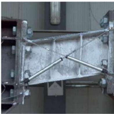
Figure 114 – Comparison of post-test deformed link and the plastic strain distribution of the numerical model at the corresponding rotation
