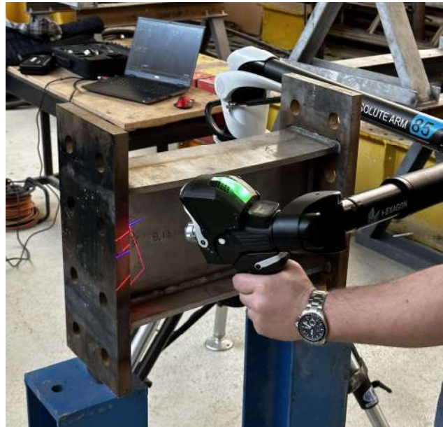
Figure 63 – Positioning of the laser probe for scanning the edges
