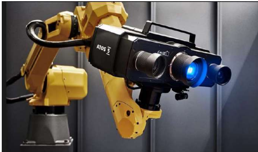
Figure 25 – Example of automated blue light scanner (Capture 3D - ATOS 5)
