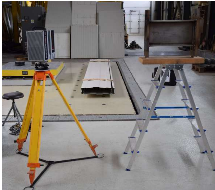
Figure 75 – General view of the LiDAR measurement set-up (b)
