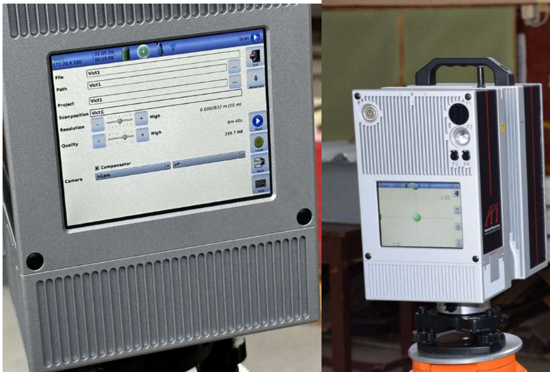
Figure 72 – Setting the resolution level (left) and calibration (right) of the LiDAR scanner
