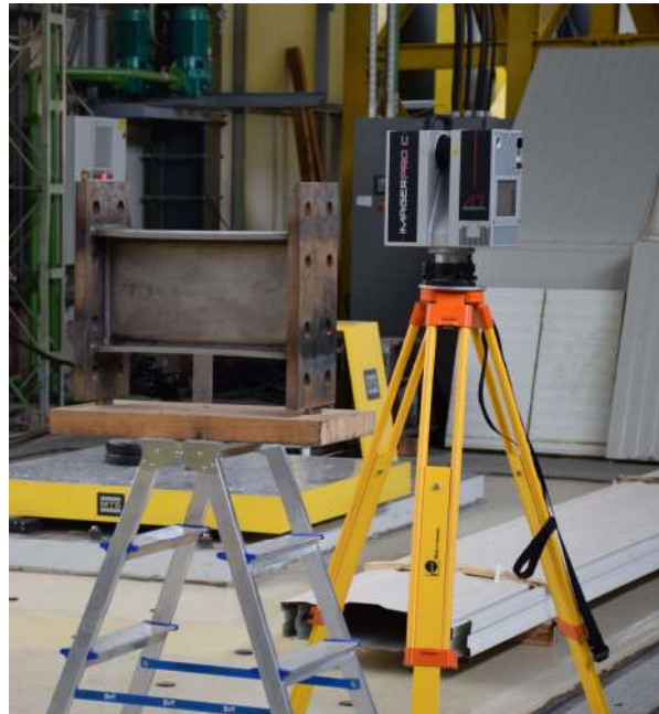
Figure 74 – General view of the LiDAR measurement set-up (a)
