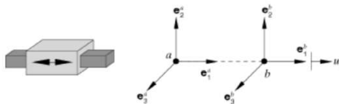
Figure 4.9: Connection type TRANSLATOR imposes kinematic constraints and uses local orientation definitions equivalent to combining connection types SLOT and ALIGN [11]
